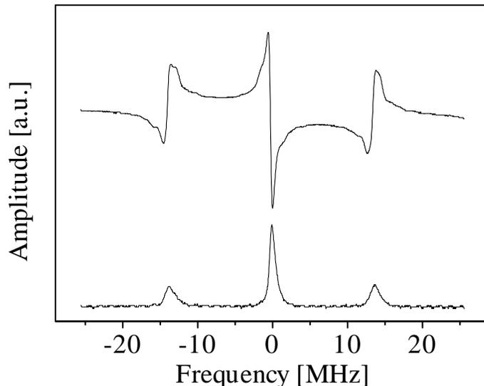
**Figure 6.14:** Scan of the laser frequency across the resonance of the cryogenically cooled cavity (lower figure). The two sidebands at  $\pm 13$  MHz are clearly visible, the finesse amounted to 11 000 in this measurement. The corresponding error signal is shown above.
