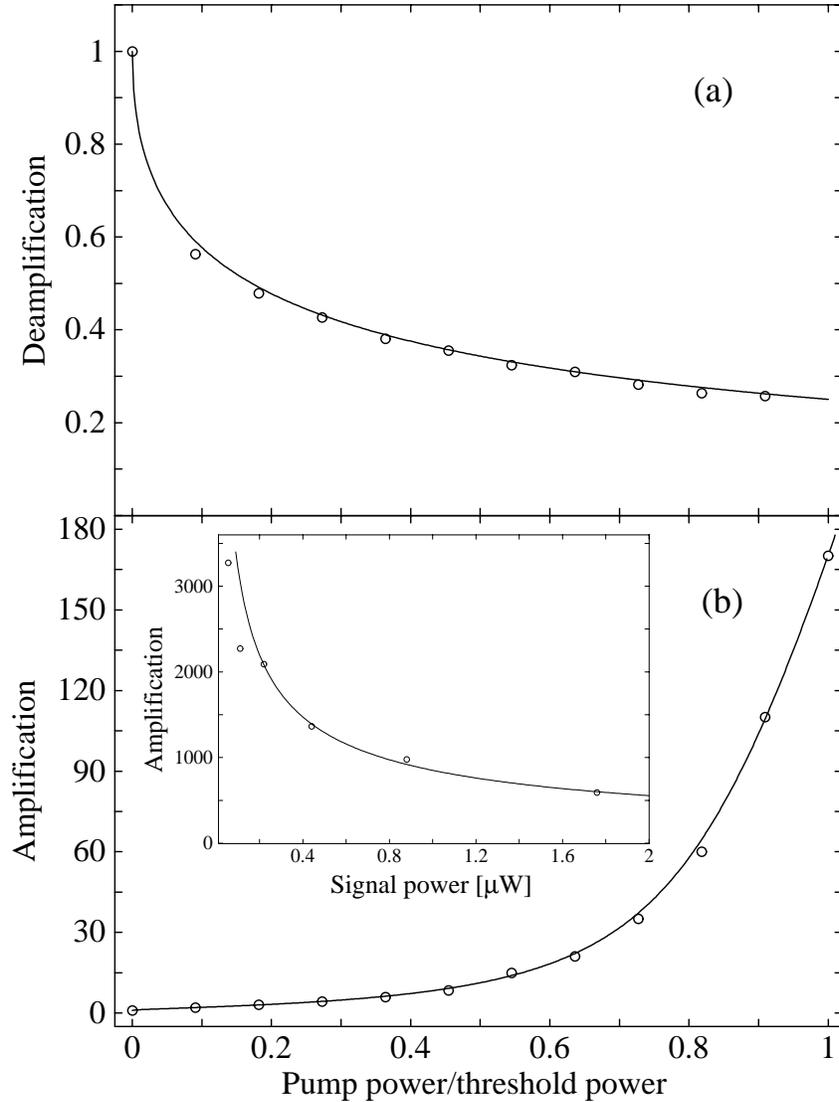
**Figure 3.5:** Parametric deamplification (a) and amplification (b) of a weak signal injected into the OPA. The signal input power in (b) amounted to  $P_{in} = 40 \mu\text{W}$ . Inset: Maximum amplification vs. signal input power at constant pump power  $P_p \approx P_{th}$ . Lines: Theory, Points: measured values.
