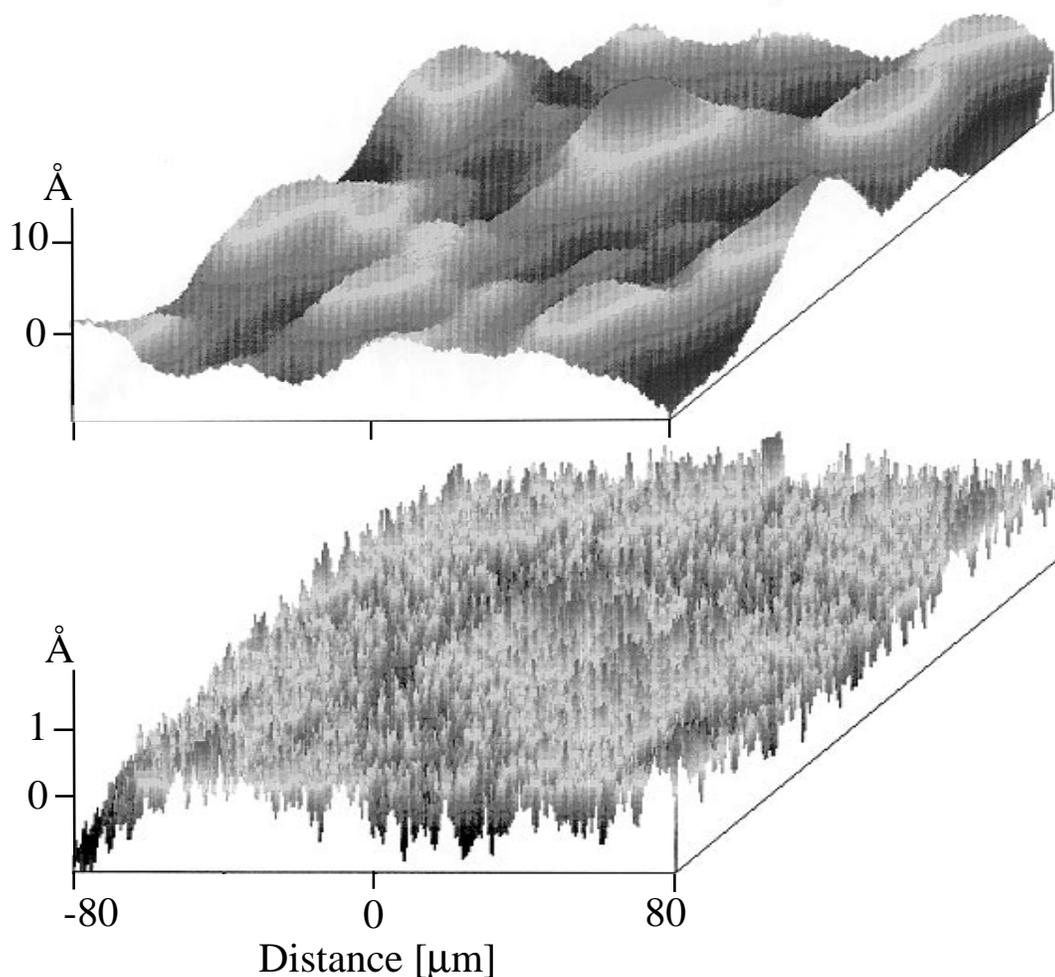
**Figure 6.11:** Surface measurements of the vane of the silicon torsional oscillator before coating (upper image) in comparison with a quartz substrate used for high finesse coatings. Both images were taken with a Micromap interferometer. The waviness of the Si-surface can clearly be seen. Note also the difference in the scaling of both plots.
