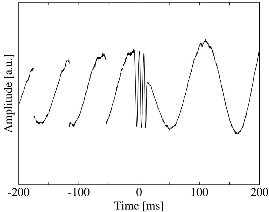
**Figure 3.29:** *Interference between the mean electric field amplitude of the degenerate OPO at threshold and a reference laser wave. Phase jumps of  $\pi$  are observable right after the start of the oscillation. Due to a change in temperature the amplitude of the OPO output rises continuously. For high amplitudes the phase remains constant. The rapid oscillation in the middle of the plot is due to the flyback of the piezo scanning the light wave's relative phase.*
