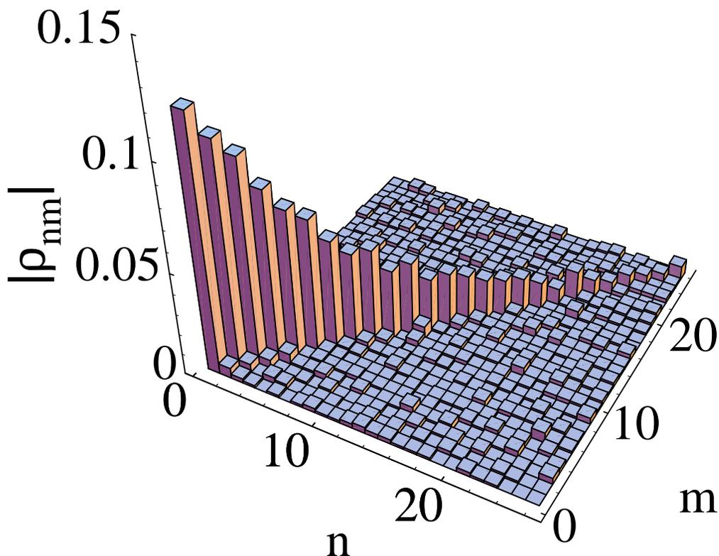
**Figure 3.35:** Reconstructed density matrix of a thermal state with  $\langle n \rangle = 6.9$  and  $\text{Tr} \rho^2 = 0.079$ , generated by random scattering via a rapidly rotating transparent wheel with a rough surface.
