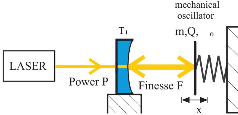
**Figure 5.1:** Sketch of the experiment consisting of a laser source and a Fabry-Perot cavity. Goal is a precision measurement of the movable mirror's position.
