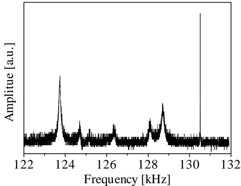
**Figure 6.10:** Spectrum of the microoscillator. The sharp narrow resonance at 130.5 kHz is due to the torsional movement of the vane. The  $Q$ -value, obtained by measuring the width of the resonance, amounted to 27 400.
