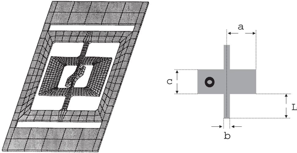
**Figure 6.2:** Left: Vane-frame torsional oscillation (exaggerated amplitude) generated by an FEM-simulation. The point off-axis where the laser beam is reflected from the coated inner vane in the cavity setup is depicted in the sketch on the right side.
