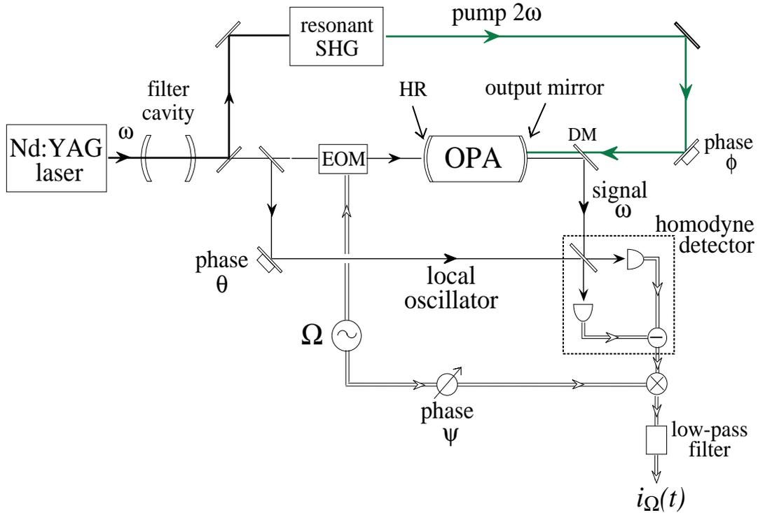
**Figure 3.1:** Experimental scheme for generating bright squeezed light and squeezed vacuum with an OPA. The electric field quadratures are measured in the homodyne detector while scanning the phase  $\theta$ . A computer performs the statistical analysis of the photocurrent  $i_{\Omega}$  and calculates the quantum states. EOM: electro-optic modulator, DM: dichroic mirror.
