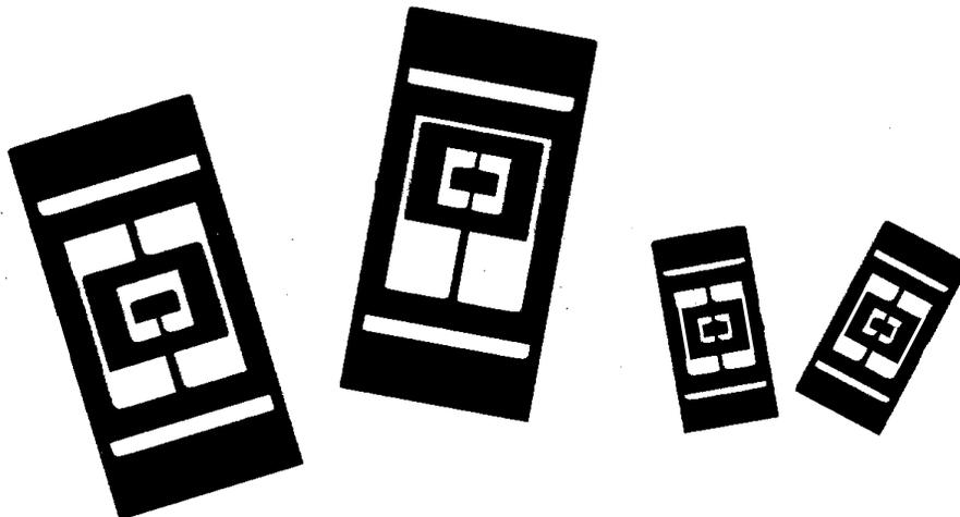
**Figure 6.5:** Lasercut oscillators of different designs. Left design: Vane held by only one bar to reduce the internal friction and to lower the resonance frequency, middle: stretched bar of decoupling frame for better isolation from the clamping area, right: test of scaling properties.
