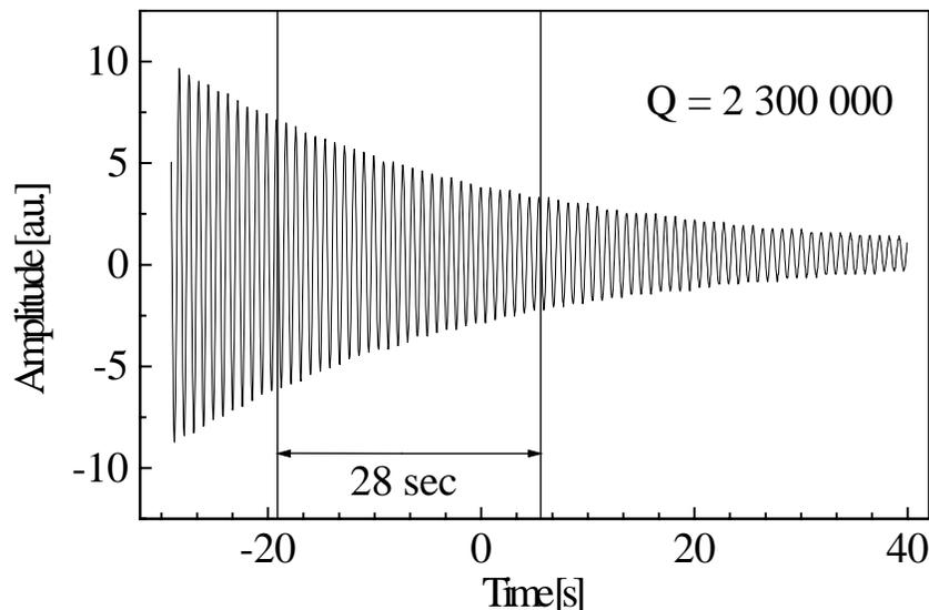
**Figure 6.3:** Typical decay time measurement at cryogenic temperatures. After the excitation via a piezoelectric transducer is switched off, the oscillator rings down in  $\approx 100$  s. The oscillation frequency shown is the beat frequency between the natural oscillation at  $\omega_0$  and the detection frequency of the lock-in amplifier.
