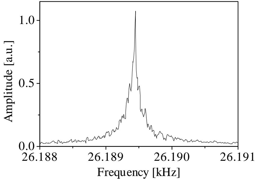
**Figure 6.16:** Linewidth of the mechanical resonance of the oscillator at room temperature, measured by reading out the error signal of the Fabry-Perot interferometer at the oscillator’s resonance. The  $Q$ -factor  $\nu/\Delta\nu$  amounted to 140 000 in this measurement. This is in agreement with decay time measurements for this oscillator, which was at room temperature exposed to a slight strain due to the fastening by 4-point glueing.
